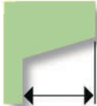
Standard (15° angle) Up to 18 mm tab extension
