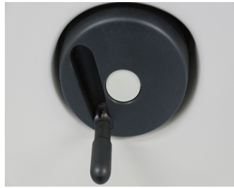
Easy format set-up with simple hand wheel activating all side lay gauges
