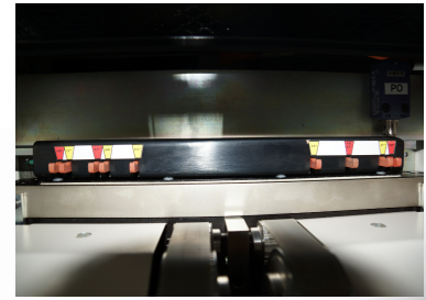
Wide range of quality punch dies with retractable pins
