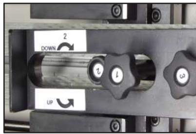
Easy format set up with setting of the pushing unit
