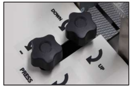
Easy format set up with setting of the clearance height and adjusting of the belt pressure
