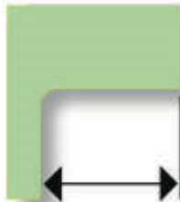
90° angle with internal round corner Up to 18 mm tab extension
