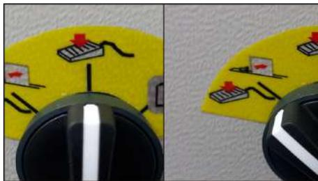
Selectable operation mode by foot pedal or by sheet presence detector
