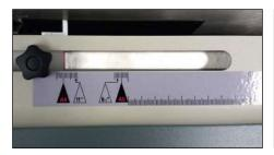
Possible adjustments according to the size of the sheets (A4, A3, ...) to be punched
