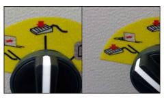
Selectable operation mode by foot pedal or by sheet presence detector
