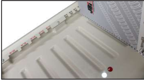
Thickness gauges to define the right Wire-O® binding diameter according to the book to bind
