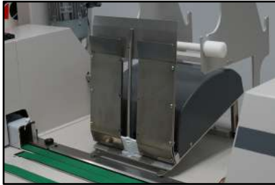
Optional automatic feeder for loose pre-formed hangers n°3 and n°7 with length from 76 mm up to 250 mm (up to 100 pieces)
